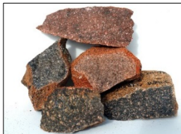
Lavas – fine grained Rhyolite (red) and Dacite (grey) with large tabular feldspar (mega) crystals
